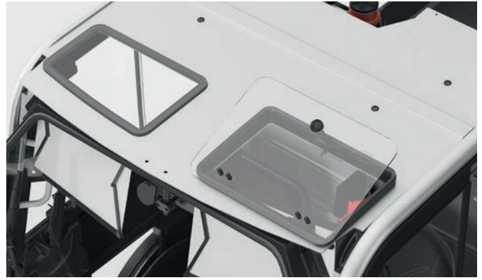
The optional roof window provides an unobstructed view upwards and additional ventilation
