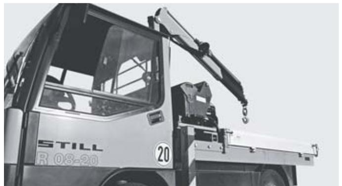
Optional built-in crane for lifting heavy loads
