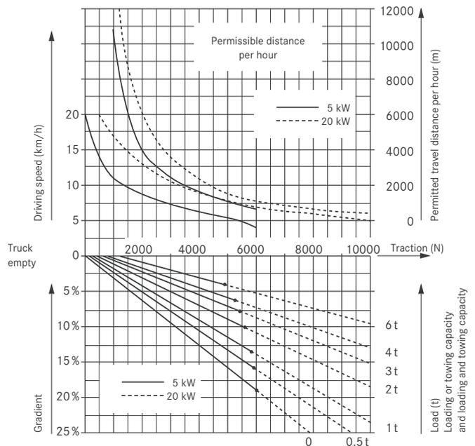
The speed and traction of the tractor can be programmed within the two curves in order to achieve the desired application. The permitted travel distance per hour is the total distance including return journeys and downhill sections (descents). The use of braked trailers is recommended if trailer weight exceeds 9 tonnes or downhill sections are to be traversed.
